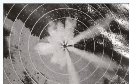
Poor injector spray pattern, from worn injector (photo taken with a microscope at nozzle point)
