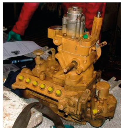
A fuel pump worn out by cavitation
